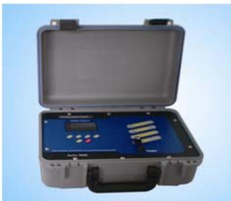
The flow calculator is equipped with a rechargeable lithium battery. This battery will require charging before initial operation. Apply 110-230VAC power, utilizing the enclosed line power cord, to the portable flow calculator for a period of 8 hours prior to using the product for the first time. The line cord connects to the socket connection located on the side of the enclosure as label.
