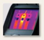
**Large and bright LCD** Sharp thermal images and easy-to-read temperature values are presented on the touch screen LCD display.
