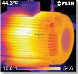
Internal winding problems and other defaults in motors and mechanical systems become clearly visible on the LCD touch screen of the FLIR E-Series.
