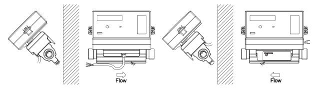
Glands and short direct sensor fitted in ULTRAFLOW® (G3/4 (R1/2) and G1 (R3/4) only)
