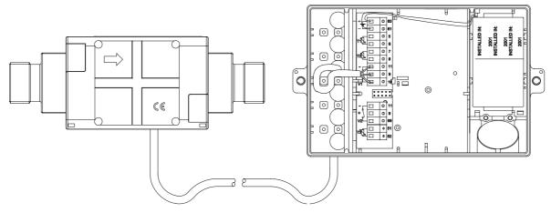
If long signal cables are used, please consider the installation carefully. There must be **at least 25 cm** between the signal cable and all other cables due to EMC.
