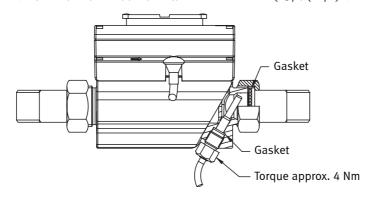
Flange meter with MULTICAL  $^{\mbox{\scriptsize @}}/\mbox{pulse}$  transmitter fitted directly on ULTRAFLOW  $^{\mbox{\scriptsize @}}.$
