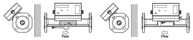
NB: For meters ≥DN100 MULTICAL® or the pulse transmitter can NOT be fitted directly on the flow part.
