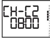
As above example, C2 relay will switch on for 8 hours. As the left side example, "08:00" shows the duration of how long C2 relay will be switched on. If switch on time is set 05:01 instead of 04:00, "04-06" interval does not have any dashes and also working time becomes 06:59 instead of 08:00.
