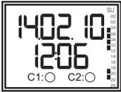
On the main menu, dashes, which exist near the numbers between '00-24', represent total working time of C1 and C2 relay.
