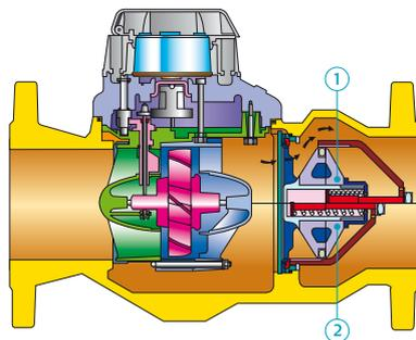
At this point, the primary meter starts to operate along with the secondary meter.
