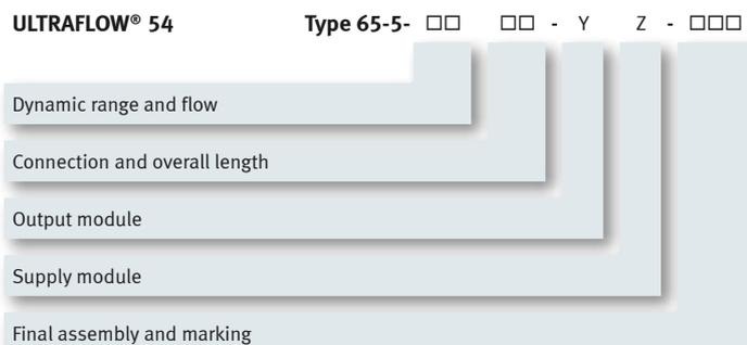
In addition to the basic variants output module (Y), supply module (Z) as well as pulse figure programming (CC) and pulse duration (E) must be selected.
