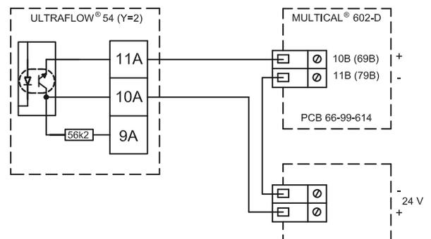
When using long signal cables, careful consideration is required in connection with installation. Due to EMC there must be a distance of min. 25 cm between signal cables and all other cables.
