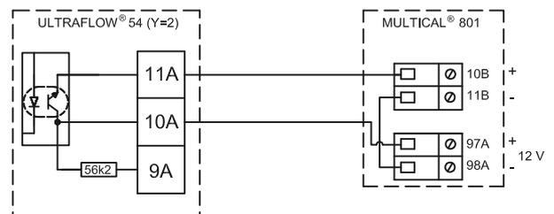
Two-wire connection, MULTICAL® 602-D via output module (Y=2) and external 24 VDC supply. Cable length up to 100 metres.
