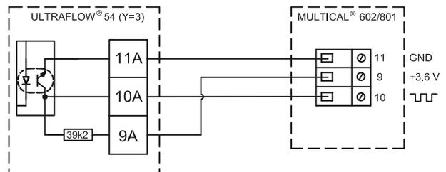
Two-wire connection, MULTICAL® 801 via output module (Y=2). Cable length up to 100 metres.
