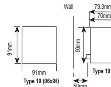
1. The device fits into a Type 19 square cut out (91 mm x 91 mm).
