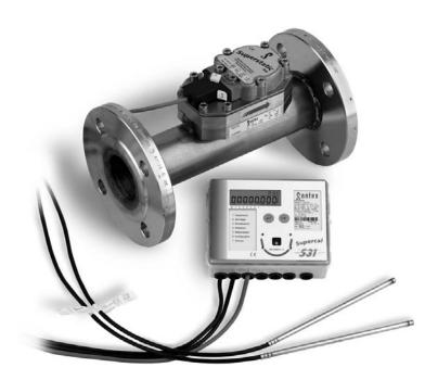
The Supestatic 440 is the heat and cooling meter with the most complete range of flows in the heat meter industry, from DN15 - DN 500 and qp 1 - qp 1500 respectively. The unique static measuring principle of fluidic oscillation without moving parts in the pipe and the robust design ensures a precise, stable and reliable measuring of flow over a long time.
