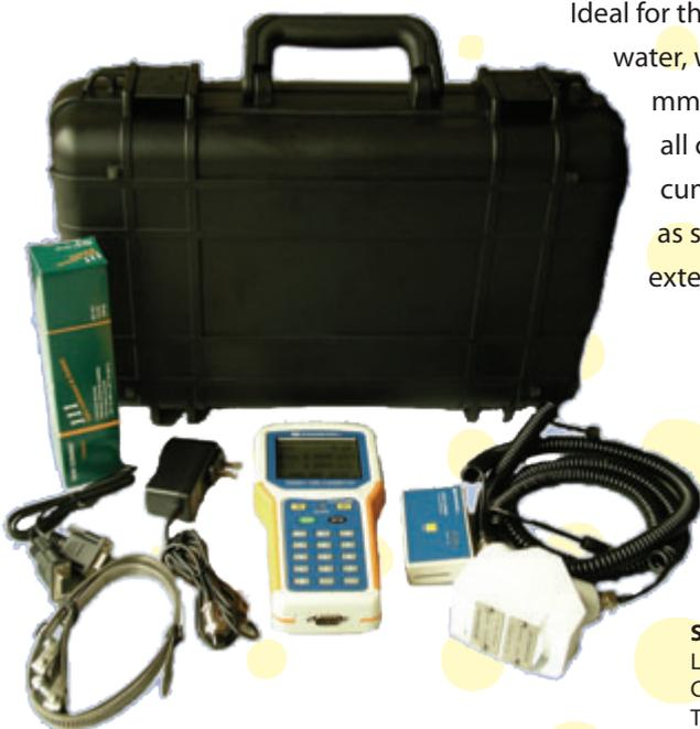
Ideal for the measurement of flows in clean, non-aerated fluids such as water, water/glycol and oils in full pipes from 1/2" to 180" (12 to 4570 mm) diameter can be measured and the ultrasonic signal penetrates all common metal and plastic pipe materials. User friendly and no cumbersome hardware, begin reading flow and gathering useful data as soon as the transducers are mounted. Connect the SL2 to external displays, recorders, data and loggers.
