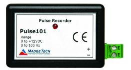
The Pulse101 is a miniature, low-cost recording device which senses pulse inputs or contact closures from external sources such as transducers and/or pulse initiators. It can collect as many as 100 pulses per second and store up to 16,383 totalized pulse counts in its non-volatile memory. Start and stop the device directly from a computer and its small size allows it to fit almost anywhere.
