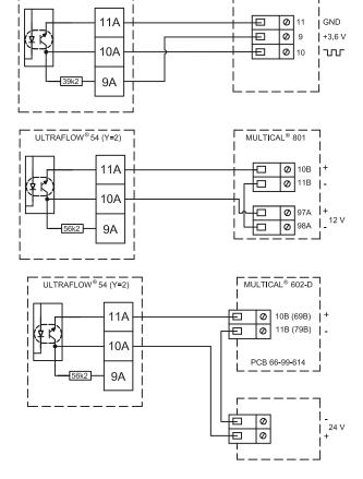
When using long signal cables, careful consideration is required in connection with installation. Due to EMC there must be a distance of min. 25 cm between signal cables and all other cables.
