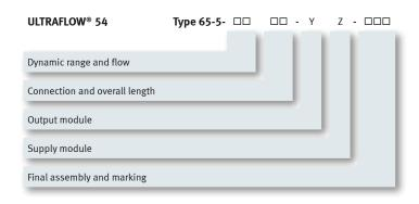
In addition to the basic variants output module (Y), supply module (Z) as well as pulse figure programming (CC) and pulse duration (E) must be selected.
