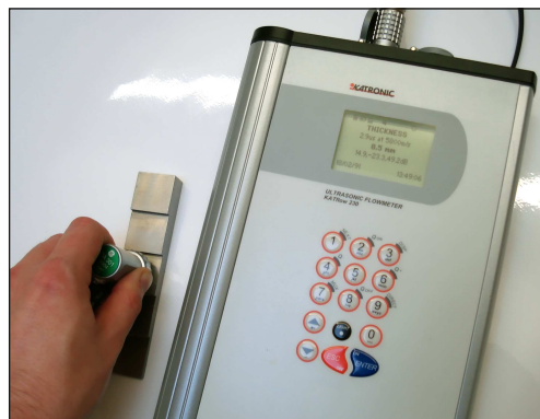
Wall thickness gauge used with KATflow 230
