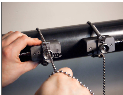
Transducers mounted using clips and chains
