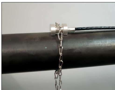
PT100 sensor fixed to pipe
