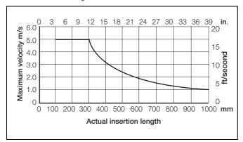
\*The graph is intended as a guide only. It is not possible to be definite as there are many effects which cannot be allowed for in such circumstances. For example, pipe vibration, fluid vibration due to pump noise, position of cable, orientation of probe entry, etc.
