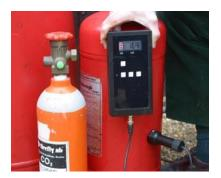
The Solenvis SL85 Portable Level Meter is a dedicated liquid level indicator for fire extinguisher systems. It is the cost effective and environmentally friendly solution for checking the liquid contents of single and multi-banked cylinder installations. It will also find the level of liquids in any single skinned metal vessel of up to1" (2.5cm) wall thickness.
